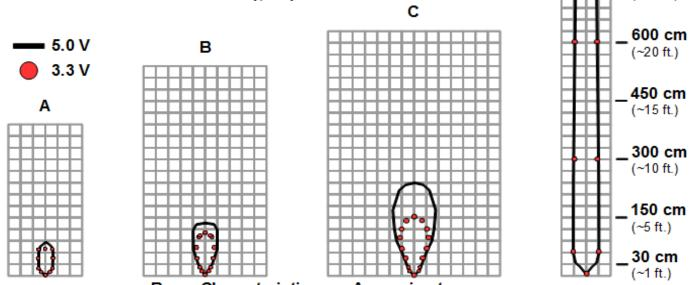
Beam Characteristics are Approximate Beam Pattern drawn to a 1:95 scale for easy comparison to our other products.
